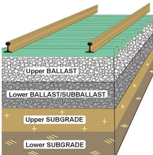
Figure 1: Idealized track substructure.
